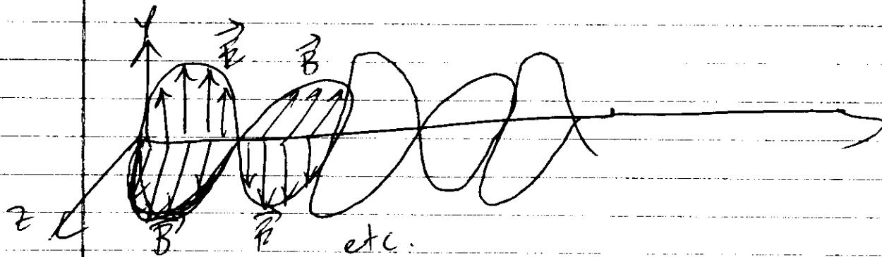
$$\frac{w}{k} = \frac{\text{frequency}}{\text{wave number}} = \text{speed of propagation}$$
