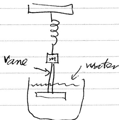
vane immersed in liquid exerts damping force
