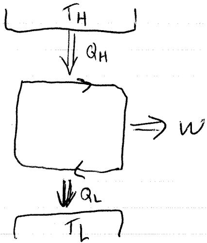
using heat to generate work, where some heat gets discarded to cold bath/reservoir.
