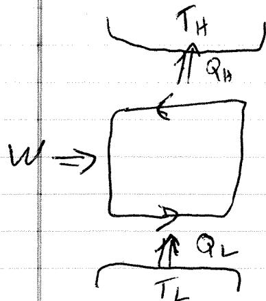
It uses work to transfer energy from a low-temperature reservoir to a high-temp reservoir
