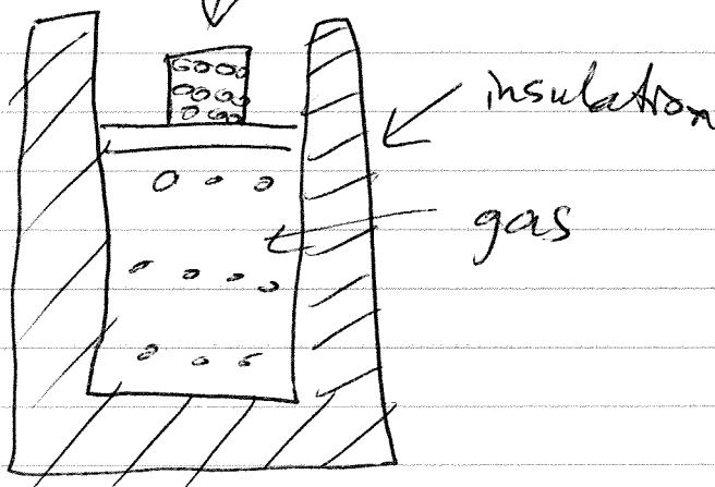
heat cannot enter ~~or leave~~ due to insulation. If we remove shot, work done by system is positive + internal energy decreases
