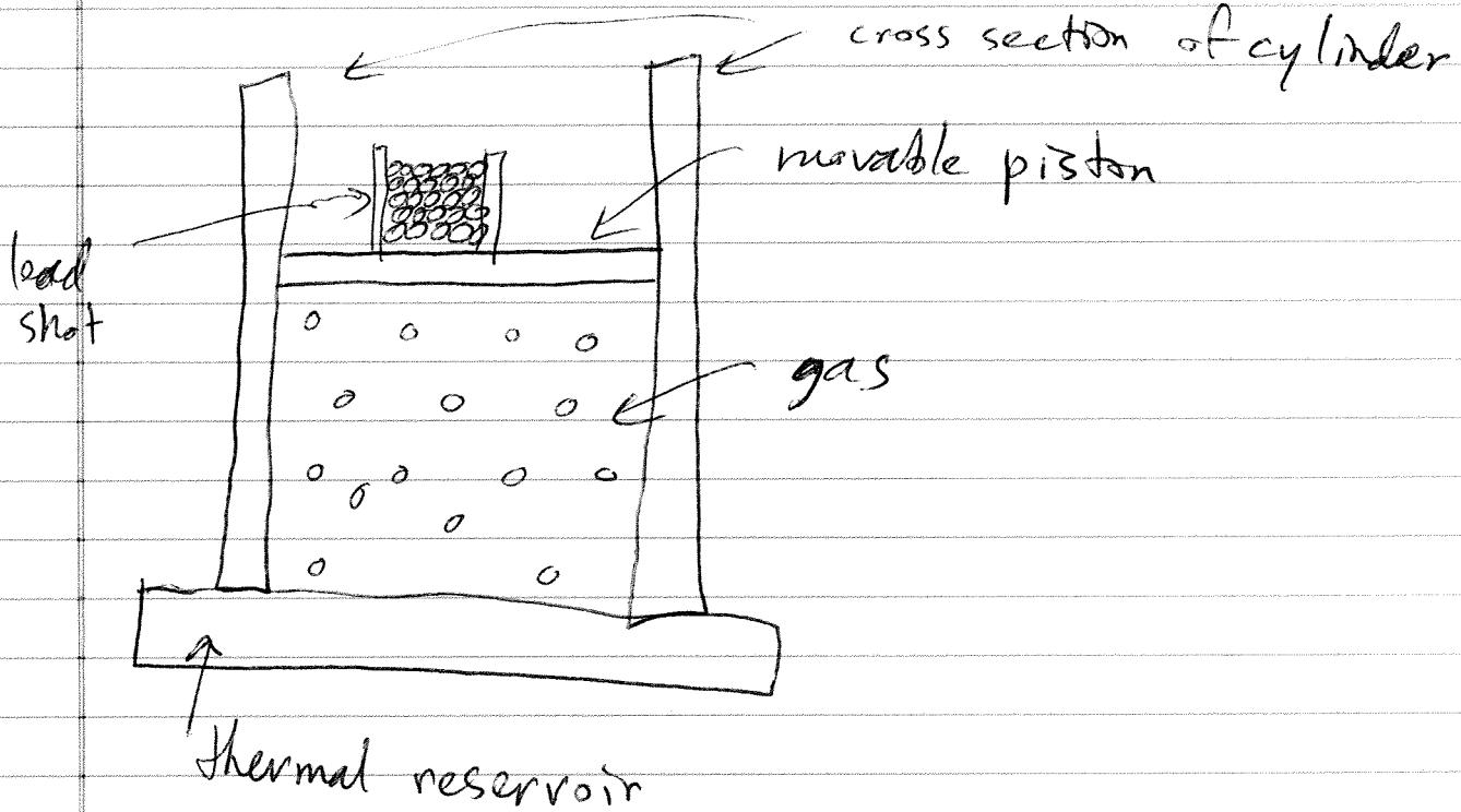
Starting out, the upward force on piston due to gas is equal to the weight of the lead shot on top
